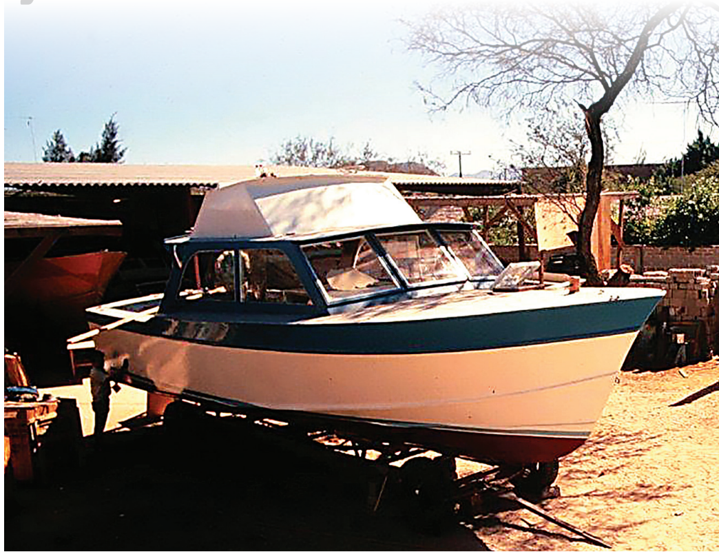
BY 1968, MAC SHROYER'S TALENT FOR BOAT BUILDING led to construction of 24-foot plywood inboard sportfishing boats for the many resort hotels springing up from Cabo San Lucas to La Paz.
